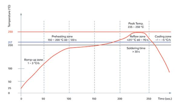
Ramp-up zone — Temp.: 25 ~ 150 °CTime: 60 ~ 90 s Ramp-up rate: 1 ~ 3 °C/s Preheating zone — Temp.: 150 ~ 200 °CTime: 60 ~ 120 s Reflow zone — Temp.: >217 °CTime: 60 ~ 90 s; Peak Temp.: 235 ~ 250 °CTime: 30 ~ 70 s Cooling zone — Peak Temp. ~ 180 °CRamp-down rate: -1 ~ -5 °C/s Solder — Sn-Ag-Cu (SAC305) lead-free solder alloy
